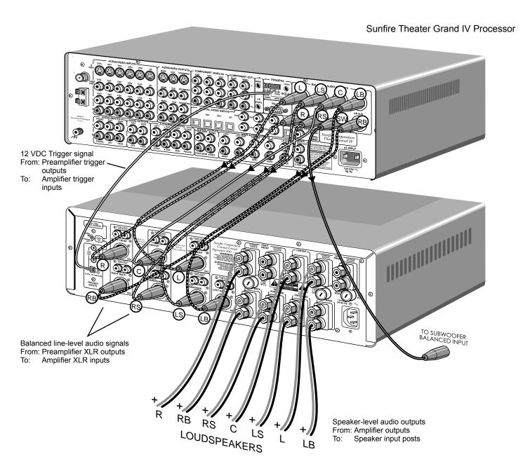
The 12 VDC trigger connection shown can be used to turn the amplifier on when the preamplifier turns on. Alternatively, you could use the amplifier's AUTO-ON switch. The amplifier will then automatically turn on when a preamp audio signal is received.
